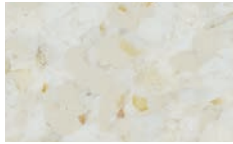
#PS2001 Marbellous Origin: refrigerators and HVAC equipment
